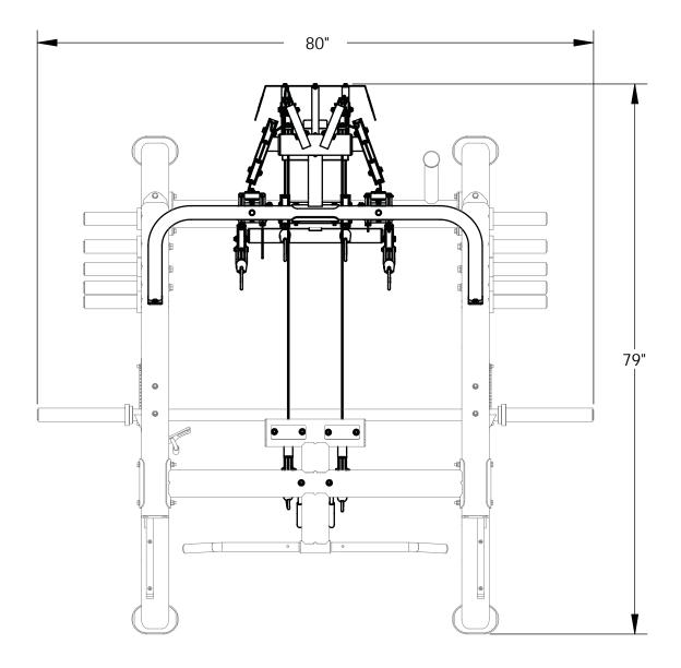
CHL-610WS Attached to CSM-600 L 79" X W 80" X H 84" CHL-610WS WEIGHT: 435 lbs. MAX-LOAD WEIGHT LIMIT 200 lbs.
