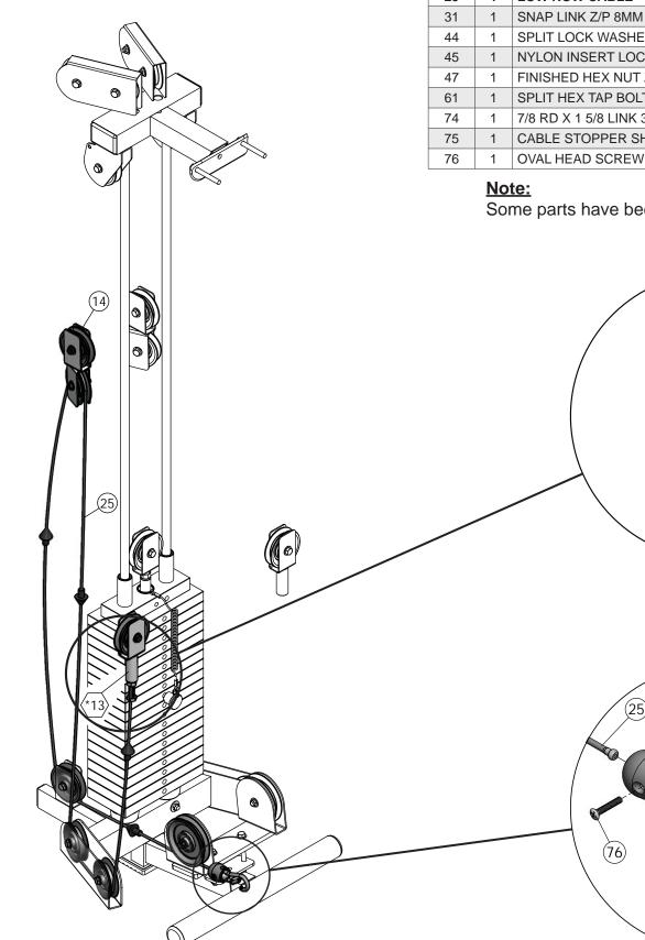
**Assembly List** Step 17 Qty. Description Item LOW ROW CABLE 25 1 SNAP LINK Z/P 8MM X 80MM SPLIT LOCK WASHER Z/P 1/2" NYLON INSERT LOCK NUT Z/P 5/16-18 FINISHED HEX NUT Z/P 1/2-13 SPLIT HEX TAP BOLT GR-5 B/O 1/2-13 X 3 1/2 7/8 RD X 1 5/8 LINK 3/16 CABLE CABLE STOPPER SHELL 1 1/2 X 1 3/4 OVAL HEAD SCREW Z/P #10-32 X 1 1/8
