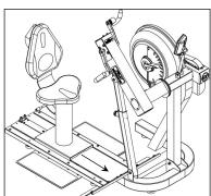
c) To remove the Seat: Lift and lower the Rear Safety lock, depress the Seat Lock Release Lever and slide the seat rearward.
