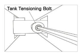
Note: Do not over tighten Tank Bolts.
