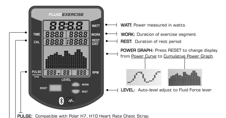
CAL: Calories burned per hour at the current Watts. Shows total calories burned when exercise is stopped.
