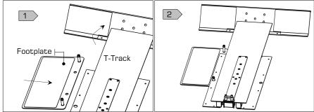
b) Mount the Left Channel over the top of the Footplate dome Bolts and then slide forward. Once Channel is properly positioned, attach to T-Track using 4x M8x45 mm Bolts[16]. Repeat this procedure to install Right Footplate and Channel.
