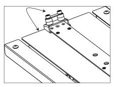
b) Seat Installation: Tilt the Seat slightly upward to allow the front Rollers to engage the channel. Then, lift the rear level and, while engaging the Seat Lock Release Lever, slide the Seat onto the Baseplate as shown.
