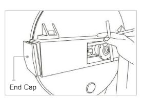
3. Loosen both the rear and front Tank Bolts slightly as shown. Remove front Rubber Belt Cover.
