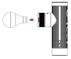
For attachment **FORK**, align the line on the attachment upward and push to connect.
