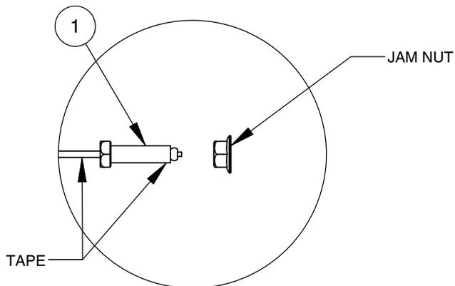
IN ORDER TO EASE FEEDING CABLE THROUGH FRAME REMOVE JAM NUT AND LIGHTLY APPLY MASKING TAPE TO BOLT (1). ONCE FINISHED FEEDING CABLE THROUGH FRAME (PG 15), REMOVE TAPE AND REPLACE JAM NUT.
