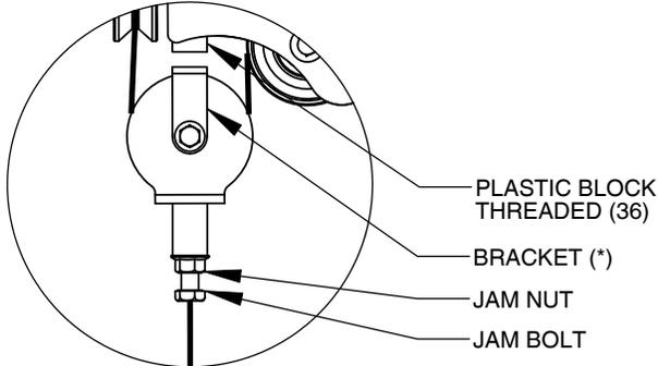
BRACKET (\*) MUST BE INSTALLED VERTICALLY, AS SHOWN TO AVOID DAMAGE TO CABLE.
