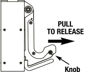
Grasp the knob firmly, lift up slightly and pull to release. Slide to your desired position before releasing knob. Make sure bar catch is securely engaged.
