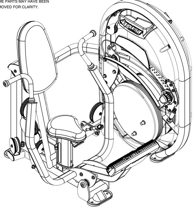
\*\*HAND TIGHTEN ALL PREVIOUSLY HAND TIGHTENED HARDWARE. NOW THAT THE CL-3301 FRAME IS COMPLETELY ASSEMBLED, TAKE TIME TO ASSURE THAT YOUR UNIT IS ASSEMBLED SQUARE AND PERPINDICULAR. IF NOT, IT MAY BE NECESSARY TO LOOSEN SOME FRAME HARDWARE TO RE-ALIGN AND THEN RE-TIGHTEN THE BOLTS\*\*
