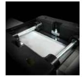
Rollers Engineering POM rollers with robust 608zz sealed cartridge bearings inserted
