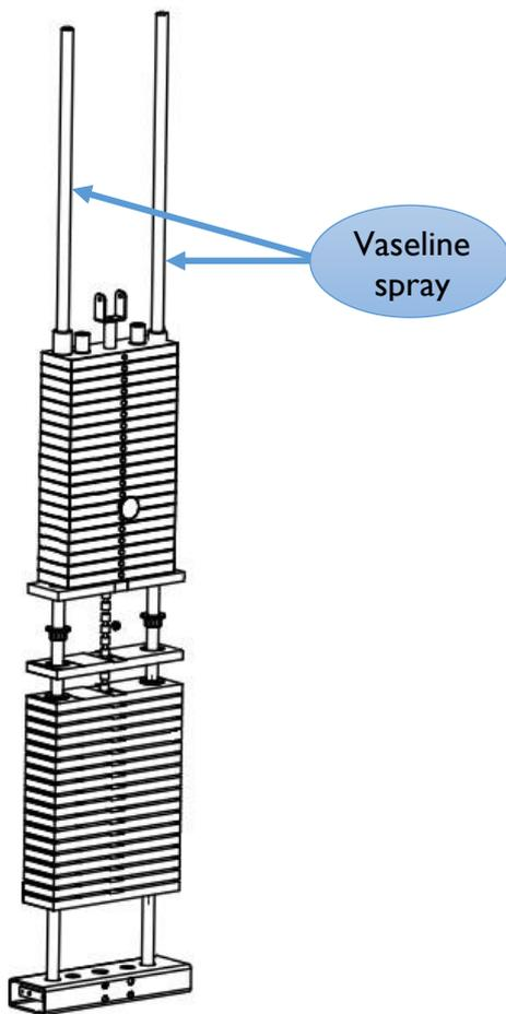
*Image 22. Lubricate the sliding bars of all Pulleys*
