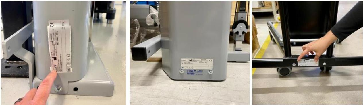
*Image 25. Location of type plate (from left: Pulley 14 & 20 and Speed Pulley 50; Speed Pulley 80 & 100 and Vertical Pull; Mobile Speed Pulley)*
