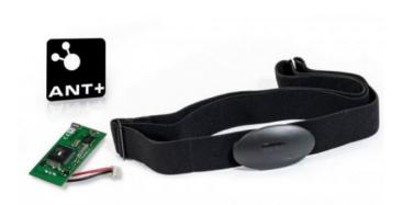
Digitally coded 2.4 Ghz connection for receiving the heart rate. The Series 4 power monitor is extended with a small circuit board that enables wireless reception from the "paired" transmitter (chest strap).
