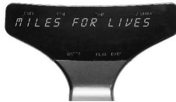
Miles For Lives is a distance program that can be used as a charity event or for a speed or endurance competition. The distance can be set from as low as 5 miles to 300 miles. The WORKOUT SUMMARY will display riders Time and Distance on a single screen to compared with the peloton.
