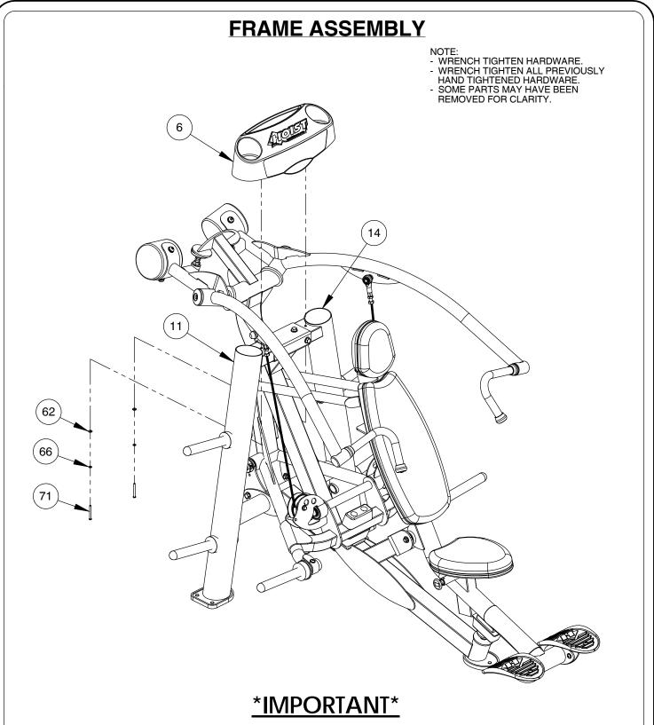
NOW THAT THE RPL-5303-A IS COMPLETELY ASSEMBLED TAKE TIME TO ASSURE THAT YOUR UNIT IS ASSEMBLED SQUARE AND PERPENDICULAR. IF NOT, IT WILL BE NECESSARY TO LOOSEN SOME FRAME HARDWARE TO RE-ALIGN THE FRAME AND RETIGHTEN BOLTS.
