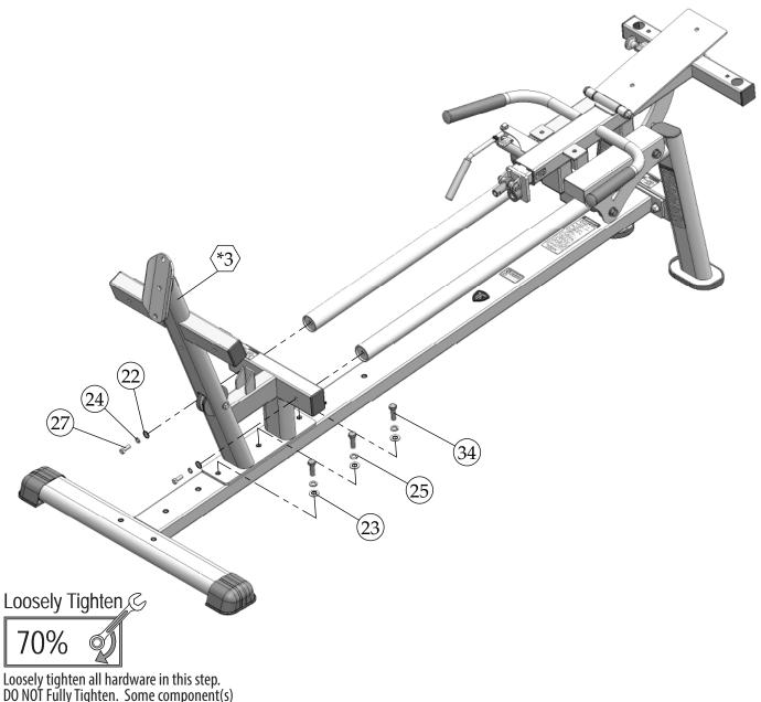
Loosely tighten all hardware in this step. DO NOT Fully Tighten. Some component(s) may need pre-assembly and or alignment during the assembly process.
