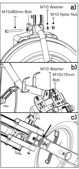
a) Carefully lower the Rower to its normal operating position to complete assembly with S-Bend installation and Frame Tensioning Bolt.
