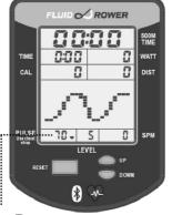
The Monitor will automatically pair with the nearest Bluetooth heart rate device.
