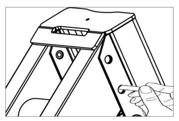
c) Secure the Rear Leg from the inside with the M6x20mm Bolts[11] and M6 Washers[16].
