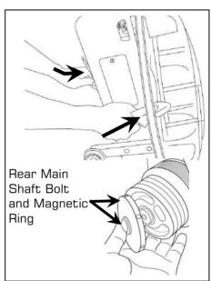
4. Next, remove the Magnetic Ring. To loosen
