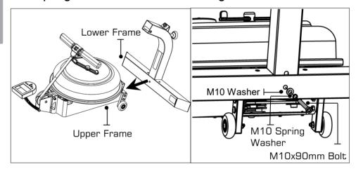
c) Install left and right side Bolts ( 2x M10x90mm Bolts [14], 2x M10 Washers[18] and 2x M10 Spring Washers [17]). Tighten all three.
