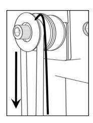
8. Upper left front to lower middle left and right Pulleys.
