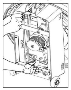
2. Move the Rowing Handle from the S-Bend to a point where it is resting on top of the Tank. This helps line up the Bungee Cord hole for easier removal/replacement. Detach Bungee Cord from lower rear attachment
