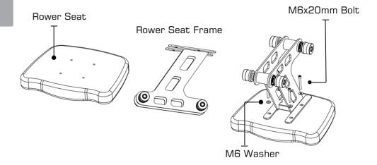
**Note:** Finished Rower Seat must be mounted exactly as shown, resembling shape of the letter 'Z'.
