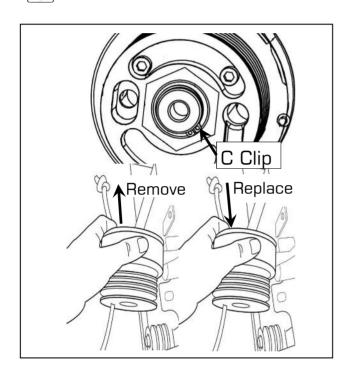
6. Move the Rowing Handle from the S-Bend to a point where it is resting on top of the Tank. This helps line up the Bungee Cord hole for easier removal/replacement. Detach Bungee Cord from lower rear attachment point.
