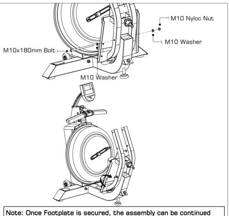
Note: Once Footplate is secured, the assembly can be continued from this position for added stability.
