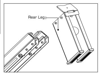
b) Install all M10x47.5mm Bolts[12] and M10 Washers [18] first from the outside to hold the Rear Leg[7] in position.
